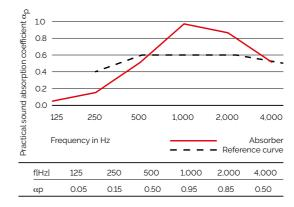
Weighted sound absorption coefficient  $\alpha_{W}$  = 0.45 Shape indicator M H
