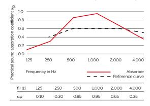
Weighted sound absorption coefficient  $\alpha_{W}$  = 0.50 Shape indicator M
