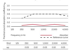
Weighted sound absorption coefficient  $\alpha_{W}$  = 0.10
