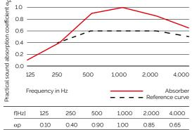
Weighted sound absorption coefficient  $\alpha_{W}$  = 0.70 Shape indicator M
