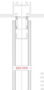
With one-sided acoustics, the partition thickness of Variflex Acoustic Light remains unchanged at 100 mm.
